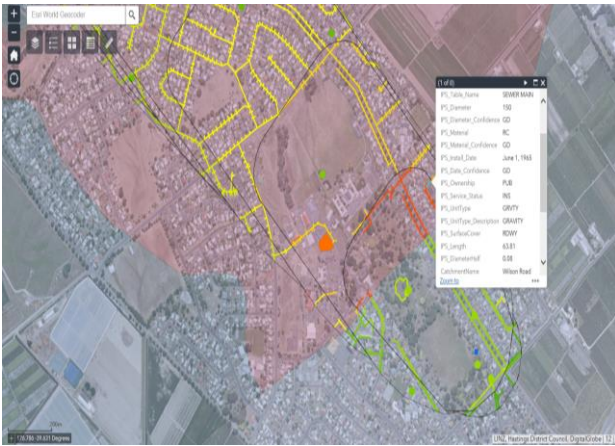
Figure 4: Shows an output of wastewater infrastructure risk. Note the impact of the relatively high aquifer vulnerability zone (refer red zone) on the final risk of the wastewater infrastructure. In this example, wastewater infrastructure located relatively close to the bore is assessed as lower risk because the aquifer has a relatively low vulnerability in that area. An absence of clay overlying the aquifer further upgradient means that wastewater infrastructure in that area poses a higher risk to the bore.
