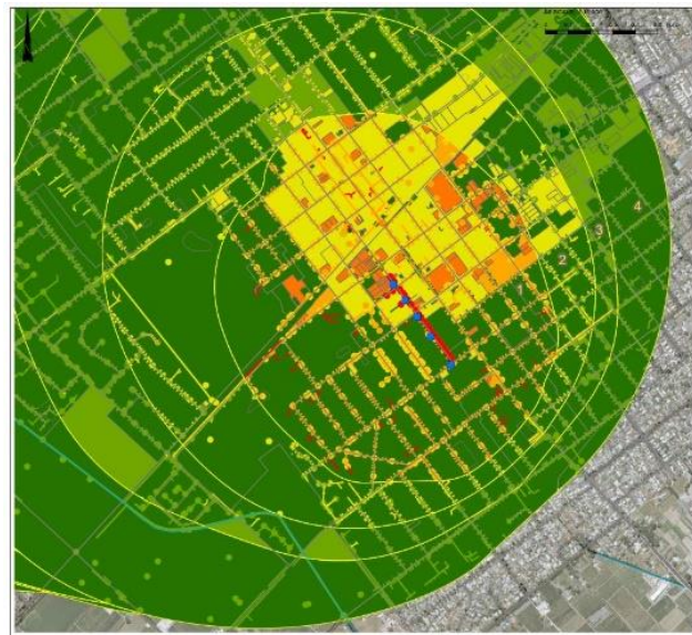
Figure 2: An example of how the tool displays relative risk at a local-scale. In this example, an alignment of abandoned former public water supply bores are assessed as presenting a very high risk to the supply (refer red symbols adjacent to the operational bores shown in blue).
