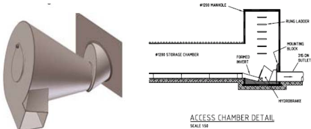
Figure 2 – Hydrobrake & Cross section of Installed Hydrobrake
